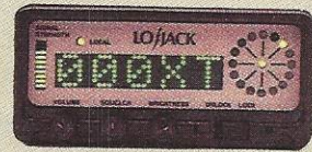
LoJack's unit (top) is hidden inside the car, and only the installer knows where. When a car is stolen, the owner calls the police, who send out a signal activating the device. Then they locate the car with a computer (bottom).
